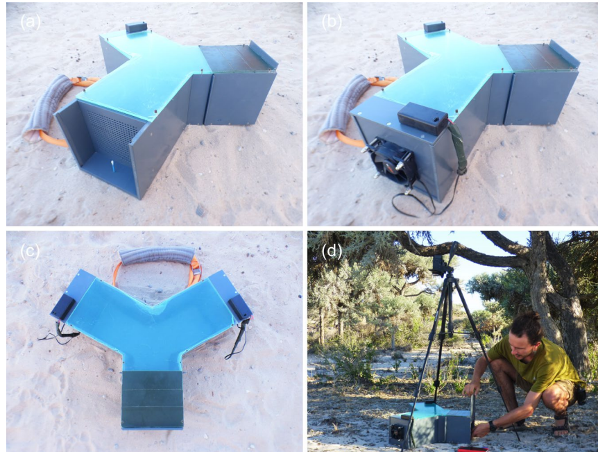
Fig. S1. Y-maze apparatus used to conduct olfactory preference trials on plover chicks in the field. The Y-maze consisted of one start arm (with opaque cover) and two test arms (with semi-transparent cover). At the end of each of the two test arms, we placed (a) a test odour (cotton swab) and (b) an electric fan powered by a battery, which circulated air from the test odour towards the inside of the maze through a perforated wall. We recorded the preference trials (c) from above, (d) using a camera mounted on a tripod, directly in the field.
